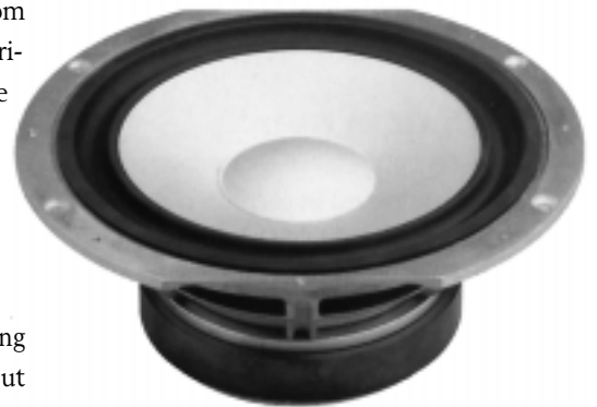
An extremely stiff aluminum diaphragm prevents unwanted resonances in the CS2.3 woofer’s frequency range.
