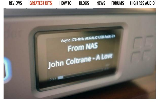
The Aurender handles DSD via DoP so the AMOLED readout reads "176.4" even though the file being sent is DSD
