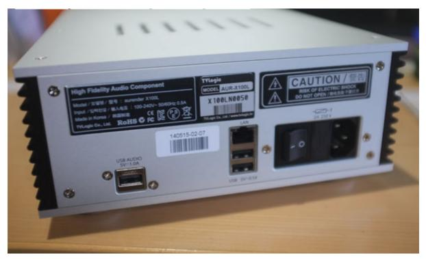
Inputs include Ethernet and 2x USB while outputs consist of a single USB socket to connect to your DAC. Aurender claims the lone USB output "is designed to deliver an exceptionally transparent audio signal free of noise and is shielded from outside electronic interference."
