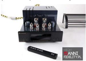
And here come an interesting operation - the signal is converted into an unbalanced one using custom, properly shielded transformers. And in this form it goes, with long interconnects, to the output tubes - 12AX7 double triodes and 12AU7, creating a gain stage and a buffer section. Both are powered by a tube, full-wave rectifier bridge based on the 5AR4.
