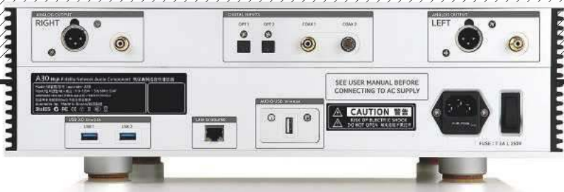
ABOVE: At the rear are pairs of coaxial (RCA and BNC) and optical S/PDIF inputs, one USB Audio Class 2.0 output and balanced (XLR) plus single-ended (RCA) analogue outs. Ethernet and two USB 3.0 ports support network connectivity and file transfers
