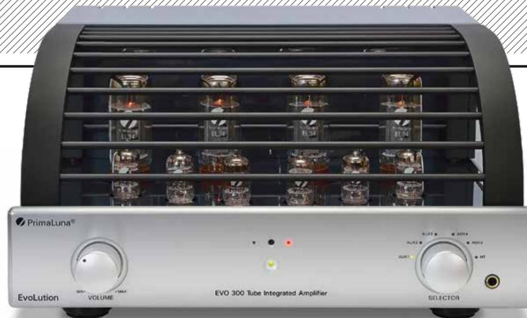
**LEFT:** The EVO chassis has rotaries for volume and input selection. Three 12AU7 double-triodes are used per channel while a wide range of power tubes are accommodated by PL's proprietary auto-biasing (EL34s are fitted here)
