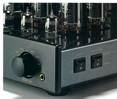
At right lie rocker switches to change bias and switch off output for headphone listening.
