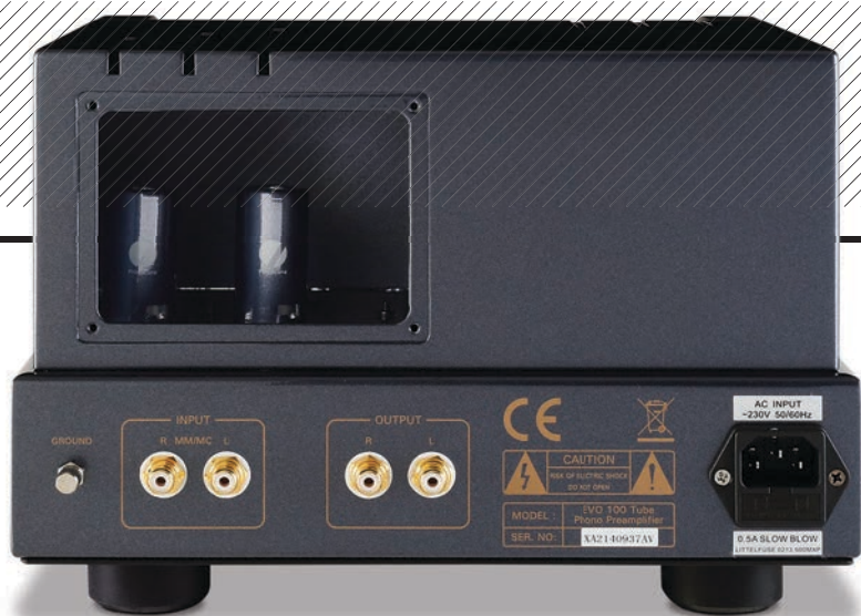
ABOVE: The EVO 100 offers one set of RCA inputs and outputs, the former switched between MM and MC via the front panel [p53]. Two 6922 double-triodes form the MC headamp, on a 'floating' PCB, seen here inside the case with the rear plate removed
